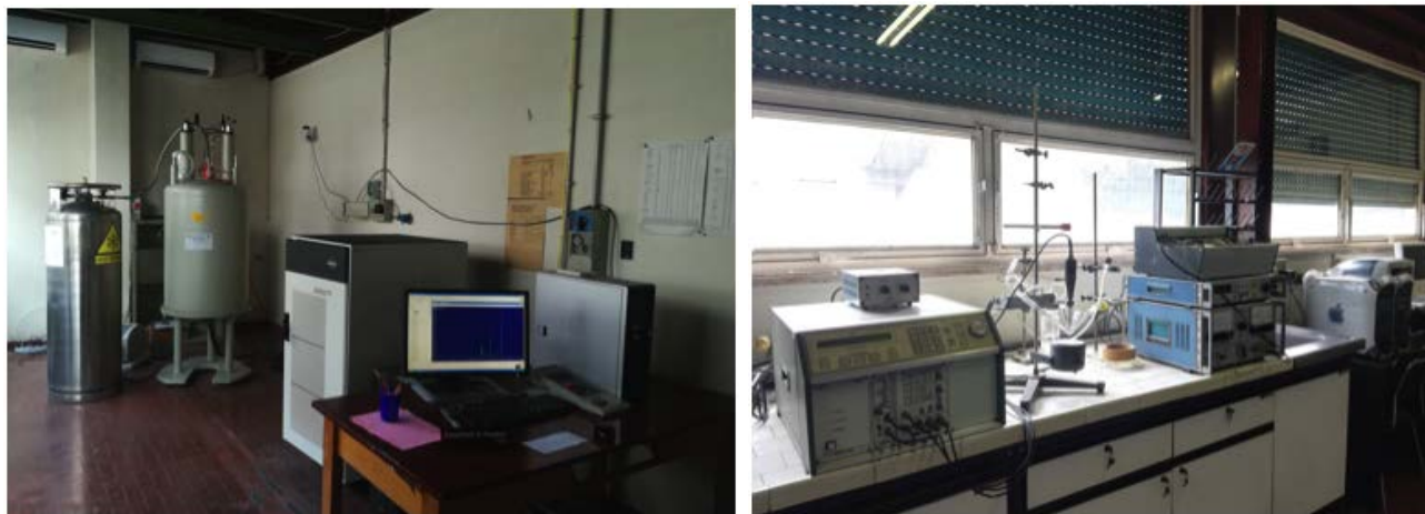
Figure 1: Left panel: NMR spectrometer; right panel: electrochemical apparatus
