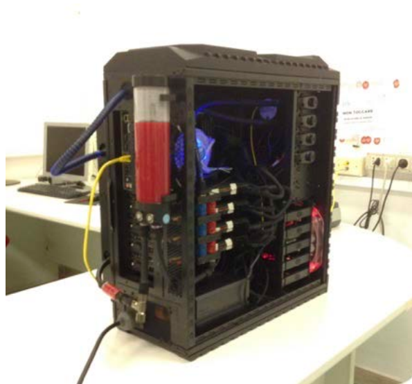
Figure 1: Closed circuit liquid cooled GPU server.
