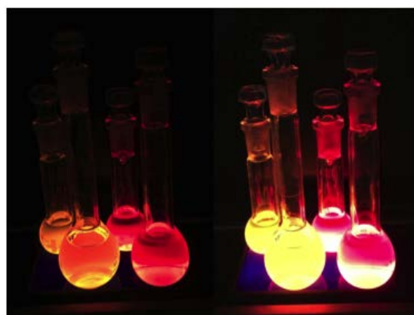
Figure 2: chloroform solutions of oligothiophenes (1 mM); UV light illumination at 254 nm (left) and at 365 nm (right).
