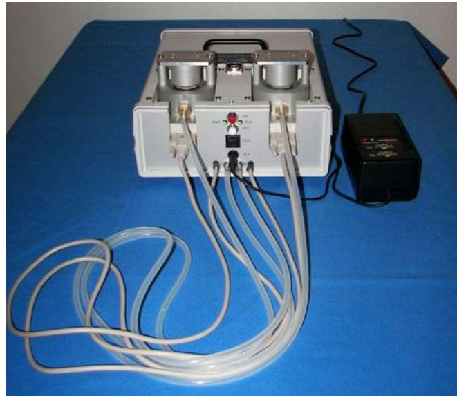
Figure 1: The Tracerlab system for measuring attached and unattached radon decay products
