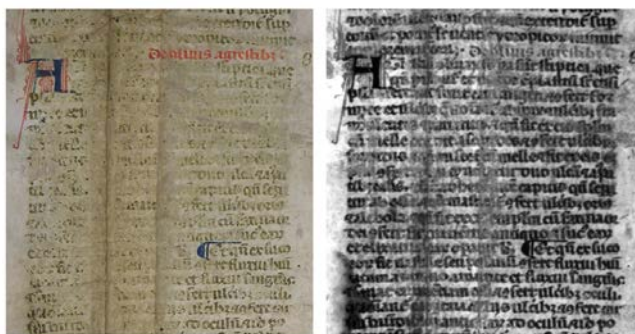
Figure 1: Digital restoring of a faded manuscript. Photography (left) and UV fluorescence image acquired using an interferential filter centered at 680 nm (right)
