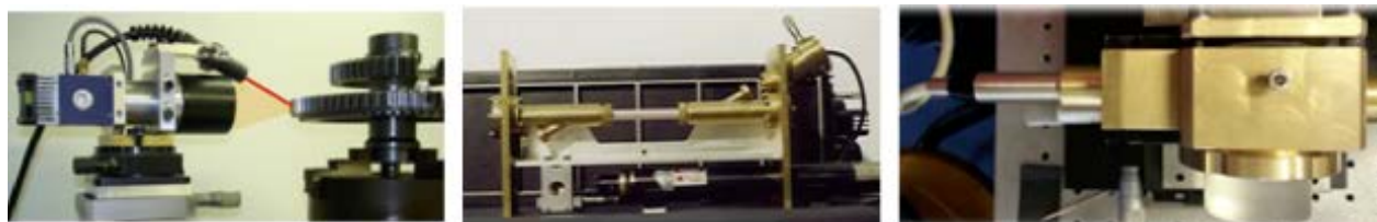
Figure 1: From left to right: Infrared radiometric set-up; photothermal detection apparatus; photoacoustic cell.
