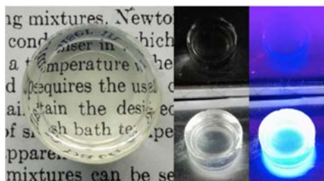
Figure 1: Plastic scintillator samples, under daylight and UV light (365 nm) illumination.
